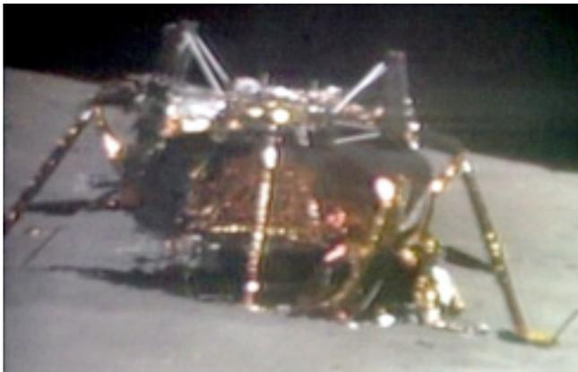
Photo of one of the Apollo Descent Stages, taken remotely by a camera left behind after the Ascent Stage had left with its two astronauts
