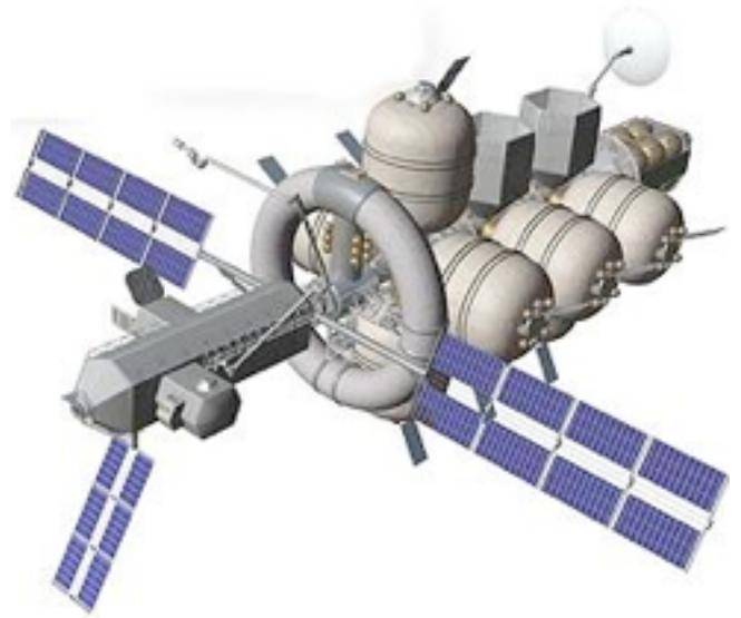
NASA concept Study for a Non-Atmospheric Universal Transport Intended for Lengthy US space eXploration, **Nautilus-X** shows several inflatable modules and a rotating torus providing artificial gravity. The dream vehicle could make round-trips to many solar system destinations
