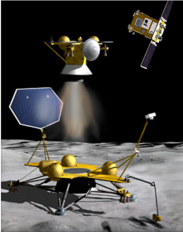
**Above:** top right **ISRO lunar Orbiter** that would maintain contact between Earth and the lander (bottom, on surface) and Sample Return vehicle (above surface, headed back)
