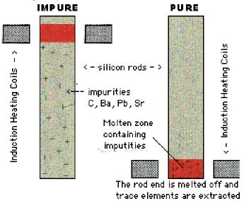
Above:Left: induction coils start to move down along the rod Above Right: The coils have reached the bottom and all the impurities have traveled to the bottom in the melt zone.
