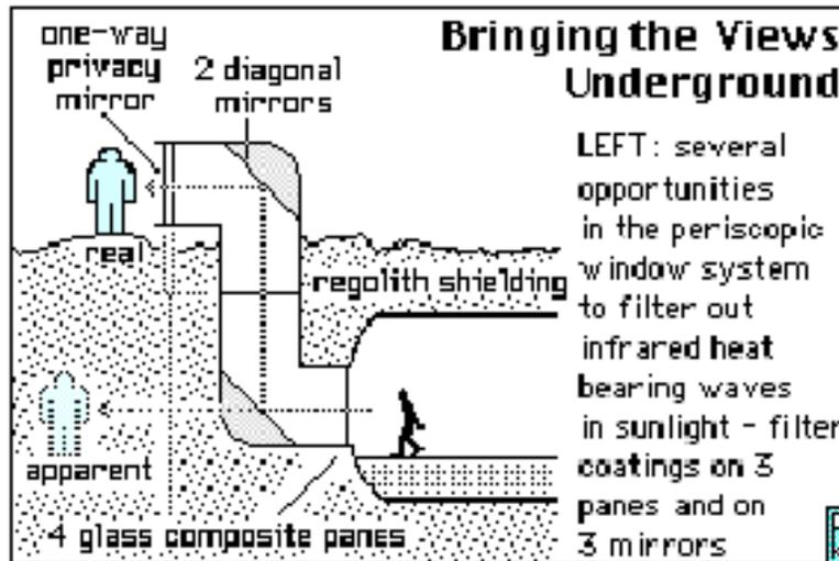
LEFT: several opportunities in the periscopic window system to filter out infrared heat bearing waves in sunlight - filter coatings on 3 panes and on 3 mirrors
