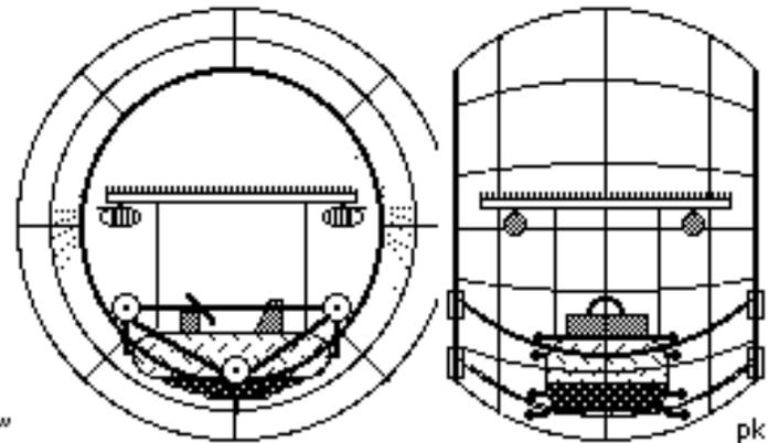
A driver pod rides the inside rails of a Lunar Squirrel Cagemobile tire-frame. Suspended above the weighted driver pod is a solar power array that also supplies some shade, and which is equipped with lights for night time operation. This unicycle can negotiate rolling terrain fairly well.
