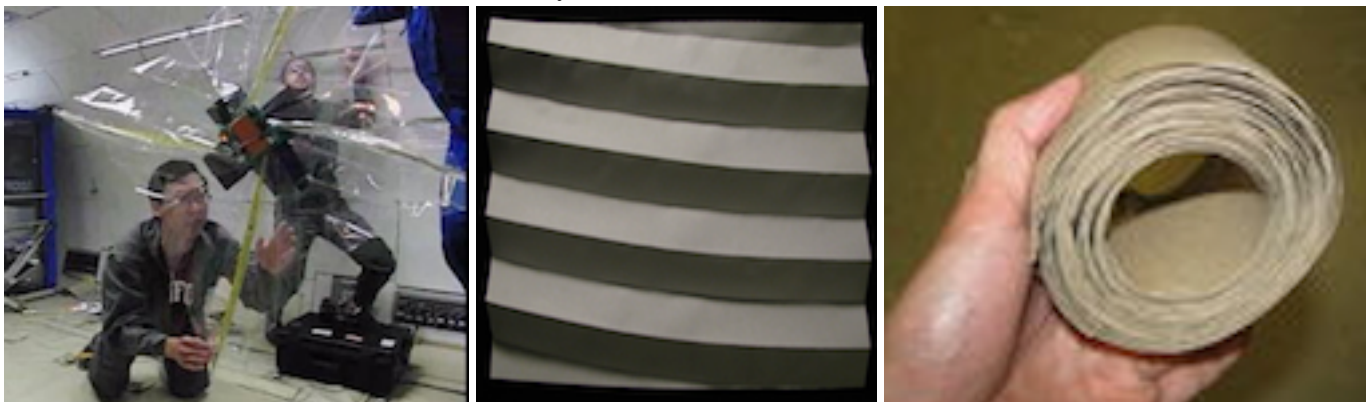
Left: deployment on Zero-G Flight Right: special way solar sail is folded to fit inside 10x10x cm cube sat
