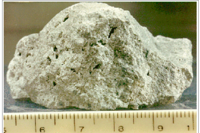
This rock is rich in KREEP Potassium (K), Rare Earth Elements (REE) and Phosphorous (P) elements rare on the Moon but abundant in the splashout from the impact that created Mare Imbrium, the nearside "Sea of Rains" - This resource may be vital to lunar industries and is not found at the poles.
