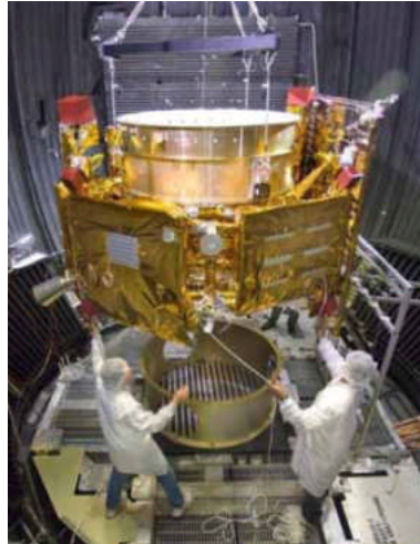
Figure 24 – LCROSS satellite in vacuum chamber testing (Bart, 2008 at Slide 11). Photo courtesy of Northrop Grumman Corp.
