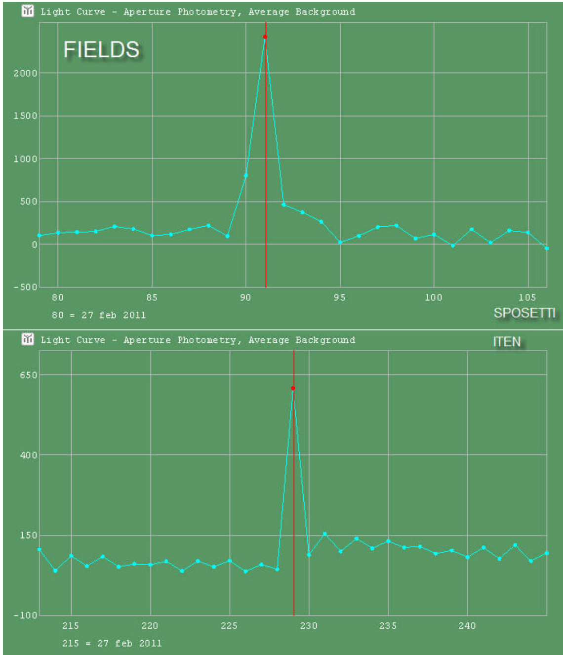
Figure 15. Light curves of the half-frames (1 half-frame = 20 ms) obtained in a circular diameter of 6 pixels (Tangra©).
