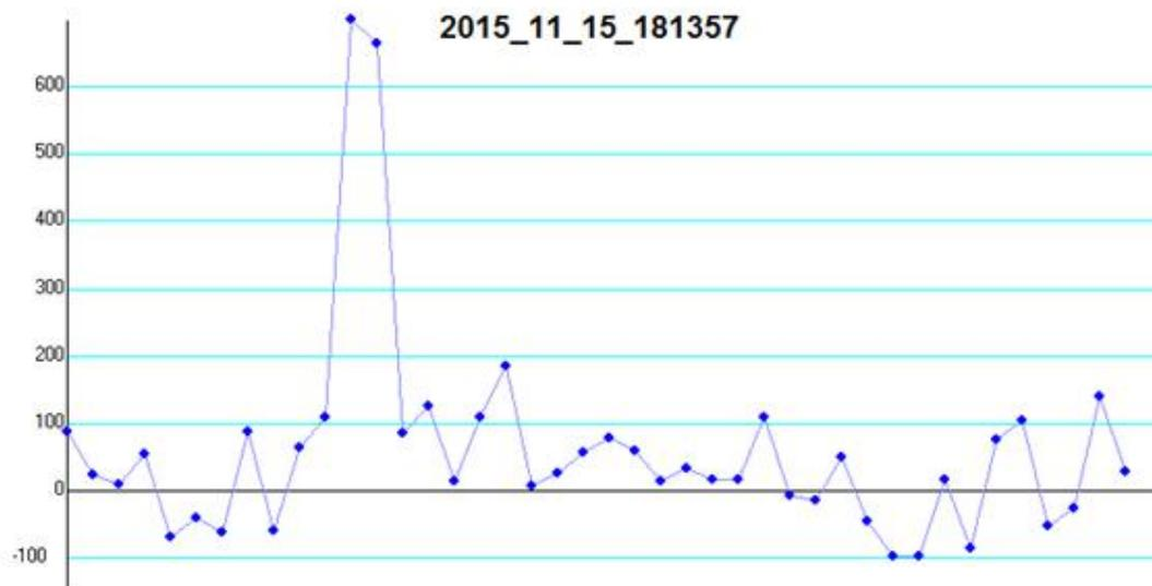
**Image 15.** Light intensity versus time of the flash N. 6. Every dot represents one field, ie. 20 ms.
