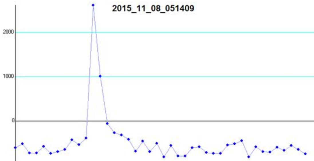
Image 13. Light intensity versus time of the flash N. 5. Every dot represents one field, ie. 20 ms.
